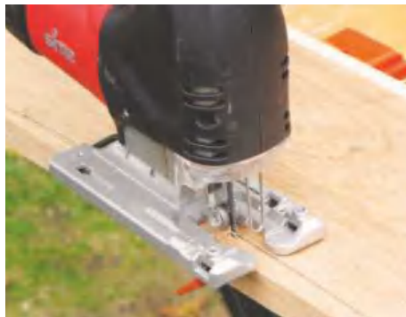
STEP 5. Next, carefully cut the curve on the waste side of the line, either on a bandsaw or with a jigsaw
